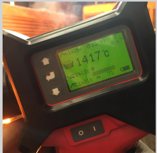
Temperature result using Cyclops L to measure melted metal pouring into the mould.
